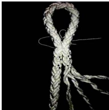
**4)** Unbraid the strands of the tail up to the first marked pair. Tape the ends of each strand pair together and cut through tape for a clean end. Continue unlaying until only the marked right-laid strand pair furthest from the eye is free.
