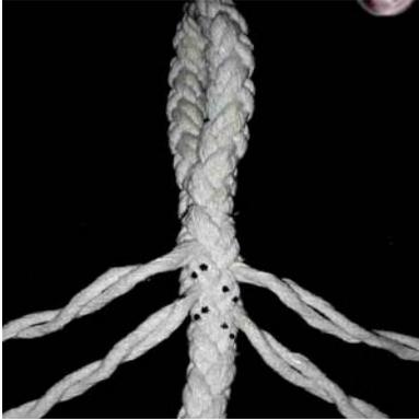
**10)** Note that all strand pairs have been tucked once now. The left-laid strands should all exit the rope on the same side. The right-laid strands should exit the rope 180° around the circumference from the left-laid strands as shown in picture on left.
