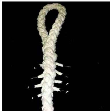
**13)** After 4\* "full" tucks and 2\* "half" tucks, the splice is nearly finished. Tape and cut the remaining strands to finish the splice. If desired, the strand ends may be "hot cut" and sealed to about 1/4 inch. The tail ends will pull closer to the braid when the splice is loaded and exercised. This retraction is normal unless it results in the loss of a "tuck".
