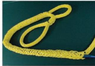
**Step 8** - Pull the tail out to the first taper cut and take the fid off. Finish cutting the marked left and right strand pairs to form the taper.
