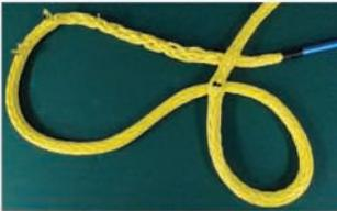
**Step 5** - Pull the taped end through until mark 2 and mark 3 meet to form the eye. Count down 3 strands and insert the fid through the rope. (Make sure you split the ends evenly on both sides again and there is no twist in the eye or splice area)
