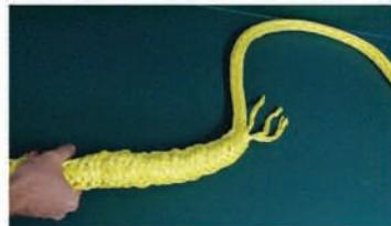
**Step 10** - Finish the splice with a whiplock.
