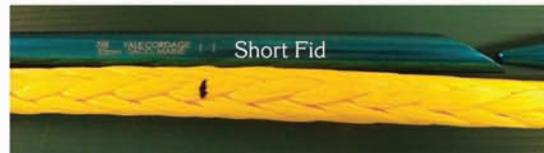
**Step 2** - Measure from mark 1 the number of fid lengths for the type of rope you are splicing and make mark 2.
