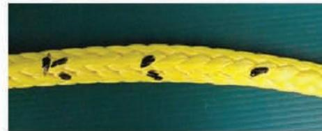
**Cut and pull out the first two strand pairs and one strand from the third pair to form the tapered end.**
