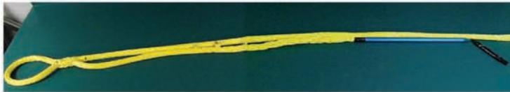
**Step 7** - Come back towards the eye and count 3 strands down and insert the fid down the center of the rope and milk the fid and tail all the way to mark 4 and exit. Make sure not to catch any of the strands.
