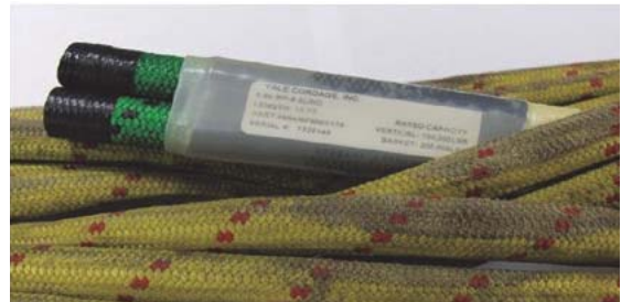
Ends can be repaired if body is not distorted
