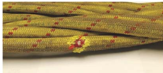
Damage Tape – Repairable
